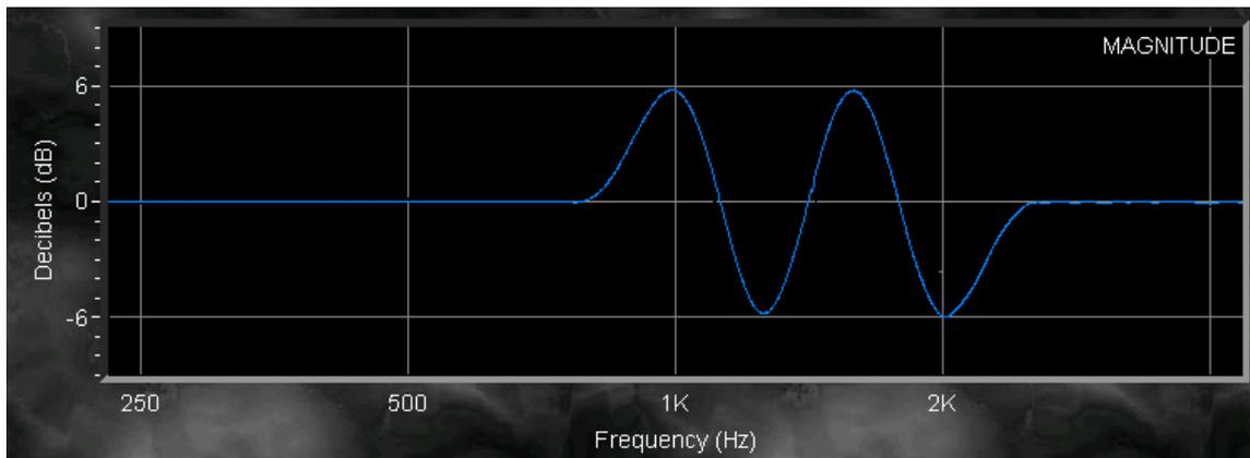
**Figure 11: Frequency response measurement of Ideal Graphic EQ**
