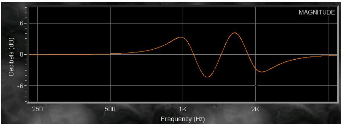
**Figure 4: Frequency response measurement of analog graphic equalizer**
