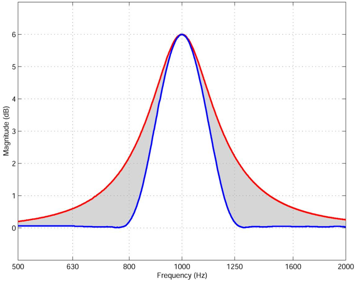
**Figure 7: Third-octave traditional parametric vs. third-octave raised cosine**
