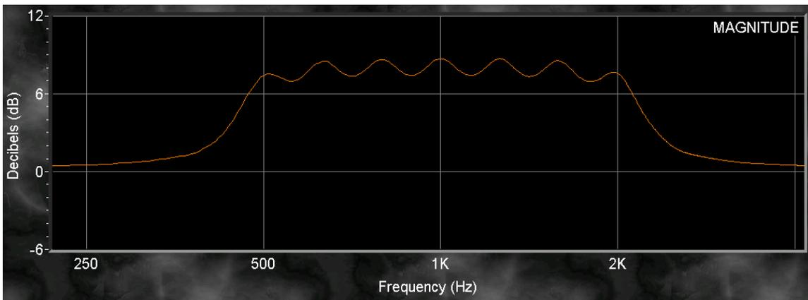
**Figure 6: Frequency response measurement of digital graphic equalizer**
