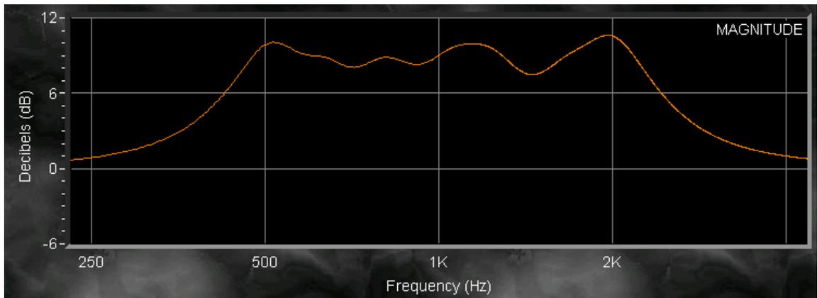
**Figure 2: Frequency response measurement of analog graphic equalizer**
