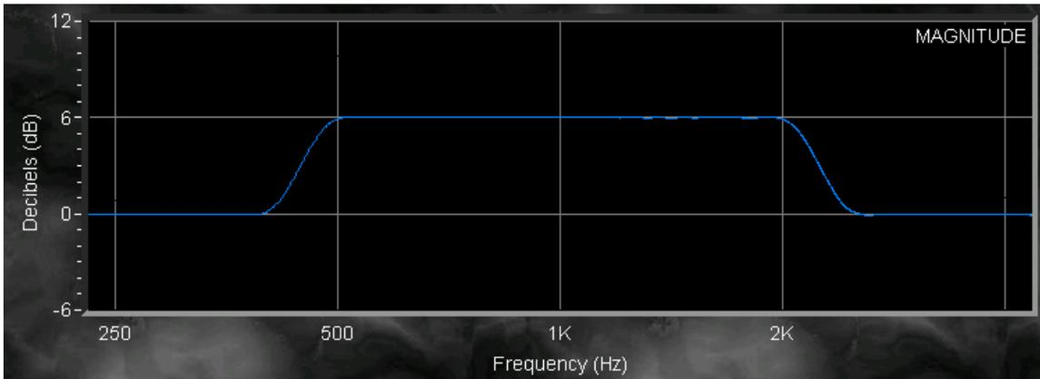
**Figure 9: Frequency response measurement of Ideal Graphic EQ**
