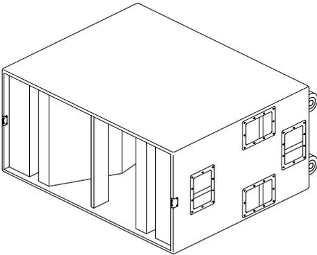
The B2-SUB is an actively driven subwoofer which uses a pair of 18" LF drivers mounted in a bandpass horn cabinet.
